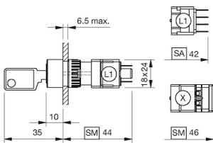
L1 = Solder/Plug-in terminal 2.8 x 0.5 mm
