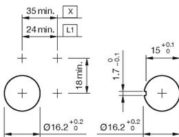
L1 = Solder/Plug-in terminal 2.8 x 0.5 mm
